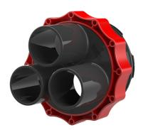
HSI 150-D1/80, 3/58 or 7/33 system cover with shrink sleeves The system covers with bayonet system are installed in the wall inserts before the cables are laid. Variants with different socket diameters are available according to requirements for sealing the cables. Hot or, alternatively, cold shrink sleeves are included in the scope of delivery. System covers with larger sockets are supplied with an additional centring strap. Empty sockets are sealed with VS blind plugs.
